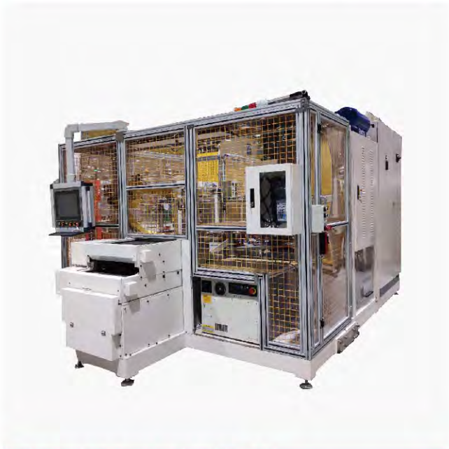
汽车座椅定位销全自动凸焊工作站 Fully Automatic Projection Welding Workstation For Car Seat Positioning Pins
